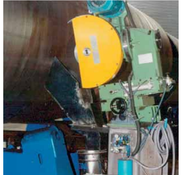
Schleifen der Wurzel aussen an Grossrohren Grinding of the root of large pipes with circumferential seam
