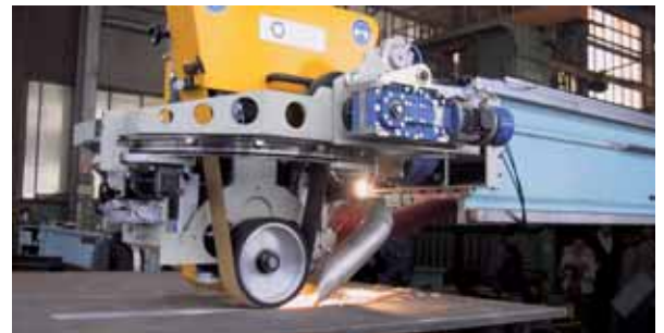
Schleifen der Wurzel aussen an Grossrohren Grinding of the root of large pipes with circumferential seam
